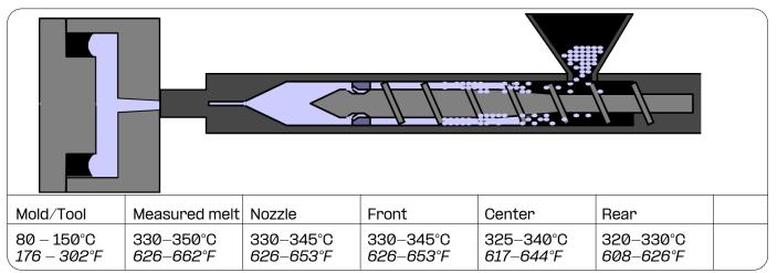
Given barrel temperature settings are for shot weights > 2 grams. For smaller shot weights (< 2 grams) barrel temperature settings are typically 5-10°C lower.
