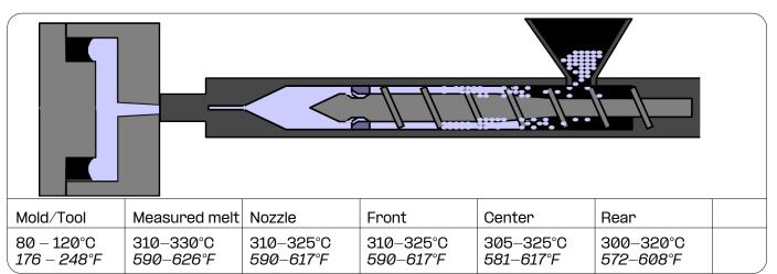
Given barrel temperature settings are for shot weights > 2 grams. For smaller shot weights (< 2 grams) barrel temperature settings are tupically 5-10°C lower.
