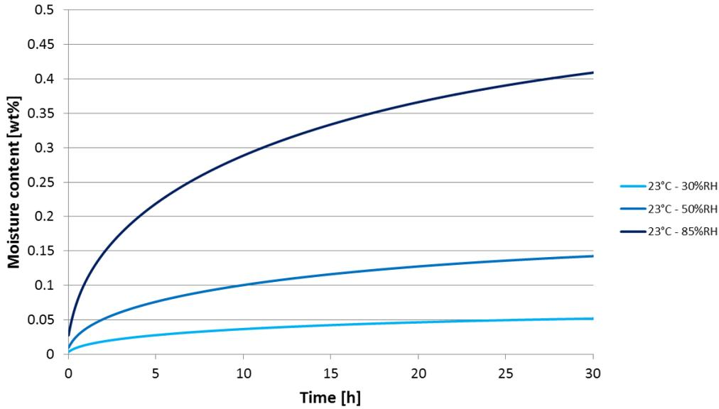
Figure 1. Moisture content as function of exposure time to ambient condition at 30-50-85 %RH. The maximum moisture content for optimal material processing is 200 ppm.
