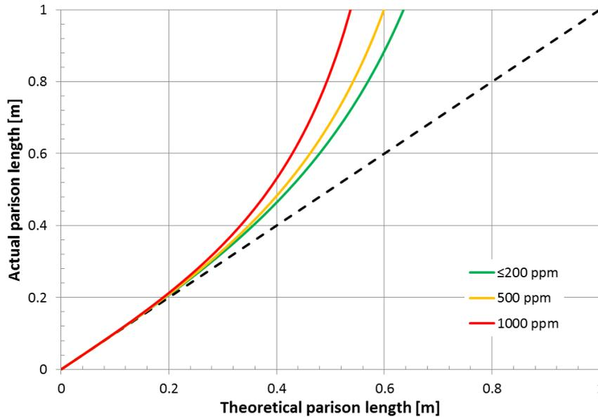
Figure 3. Loss of sagging performance in relation to moisture content of Arnitel processed at 230°C. The dashed line shows the parison extrusion without sagging.
