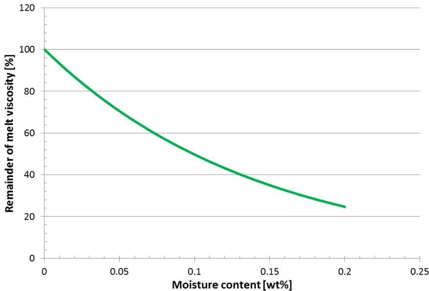
*Figure 2. Loss in melt viscosity in relation to moisture content of Arnitel at 230 °C. It is advised to process Arnitel at moisture content values  $\leq 200$  ppm. For instance, processing at 0.1 wt% moisture content will decrease melt viscosity by 50% of its initial value.*
